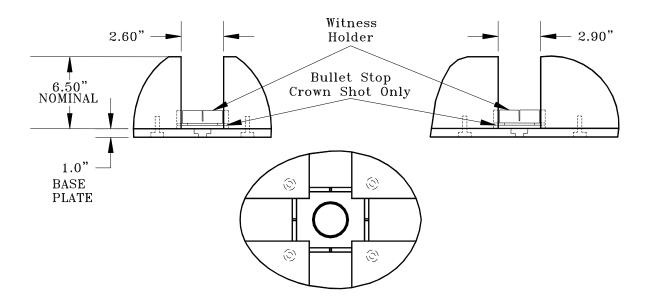
Figure 2A: Headform Configured for Penetration Testing
