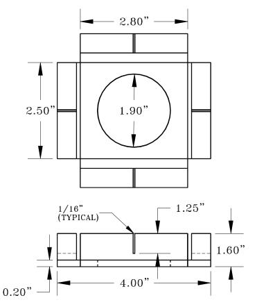
Figure 4: Penetration Test Witness Panel Holder (Mild Steel)
