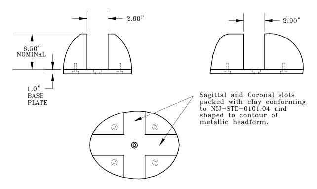
Figure 2B: Headform Configured for Deformation Testing
